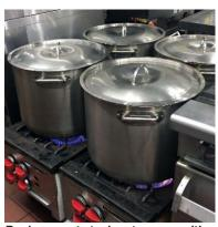
Replacement stock pot ranges with finned-bottom pots for improved heat transfer.
