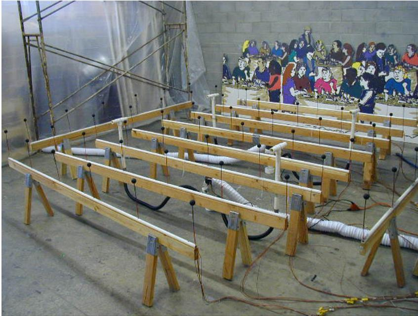
Figure 1. Globe thermometer array.
