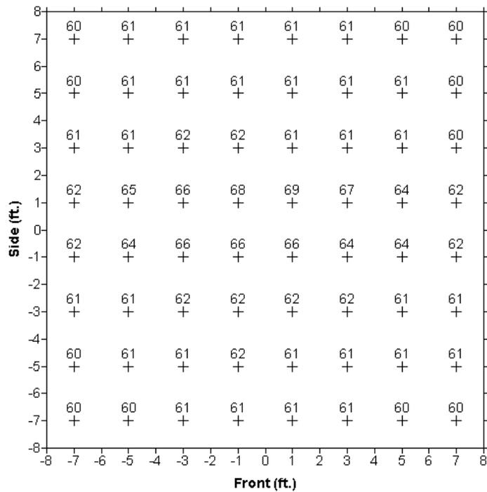
Figure 3. Test #2 normalized mean radiant temperatures.
