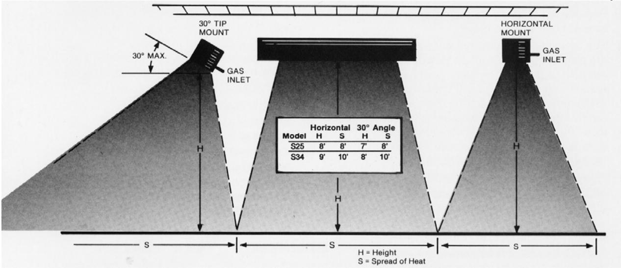
SUNPAK will raise the comfort level 5-10° Fahrenheit outdoors. The above coverage table was based on still breeze conditions. Under windy conditions more heat will be required. It is recommended that a windswept patio be designed with wind breaks to stabilize the patio environment. Wind breaks shall NOT interfere with the ventilation of combustion air requirement of the heater(s).
