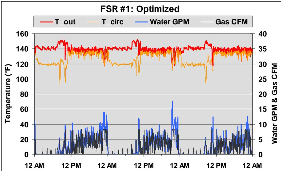
Figure 3. FSR #1 - Typical Optimized Operating Profile
