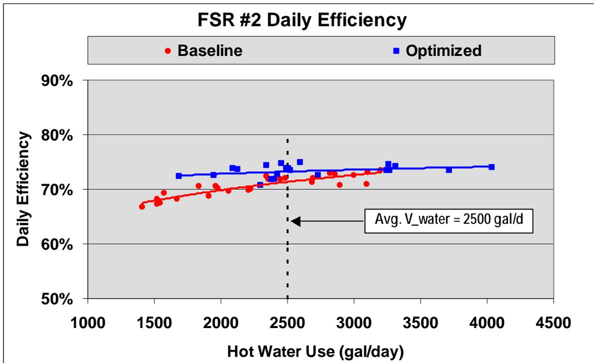
Figure 8. FSR #2 - Daily Efficiency versus Hot Water Use
