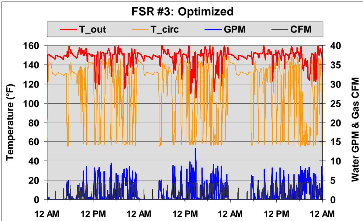
Figure 11. FSR #3 - Typical Optimized Operating Profile
