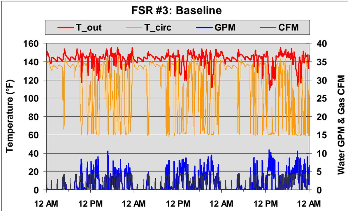
Figure 10. FSR #3 - Typical Baseline Operating Profile
