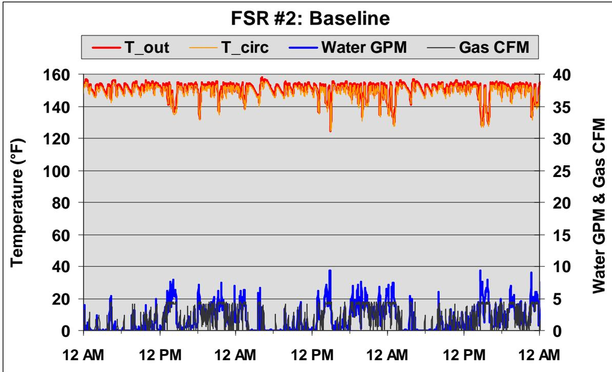
Figure 6. FSR #2 - Typical Baseline Operating Profile
