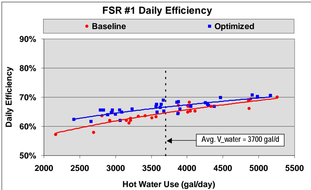
Figure 4. FSR #1 - Daily Efficiency versus Hot Water Use
