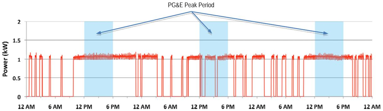
**Figure 9. Replacement Ice Machine Power Profile: Load Shifted Operation.**
