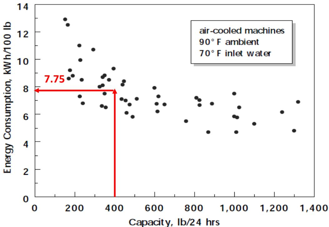
**Figure 2. Energy Use vs Ice Harvest Rate for Air Cooled, Cube Type Ice Machines (2012 AHRI Data – FSTC Analysis)**
