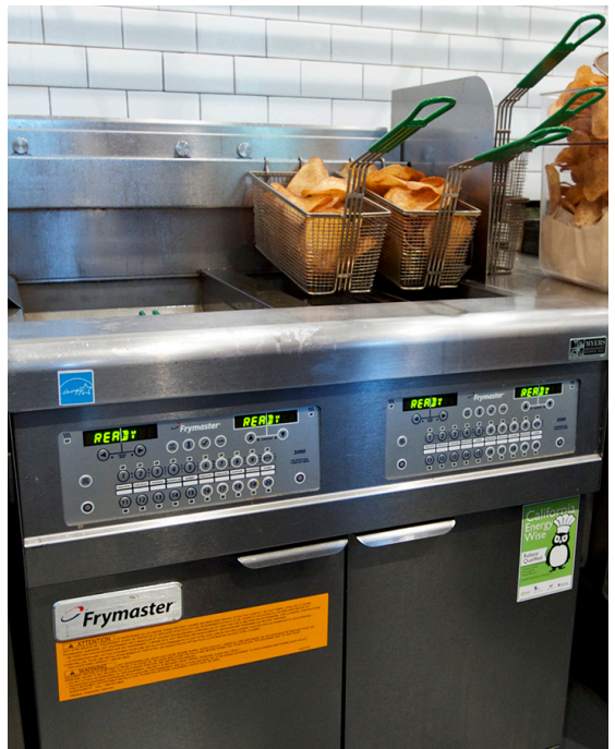
Frymaster Fryer — Double-vat, Oil Conserving Fryer (OCF) with built-in automatic oil filtration, programmable controls, and Oil Attendant®.
