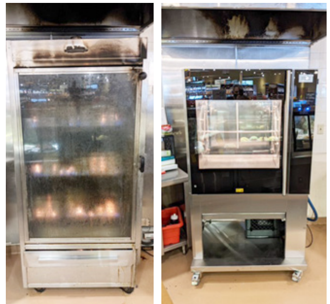
Original continuous rotisserie oven (left) and replacement Fri-Jado TDR7 batch rotisserie oven (right).
