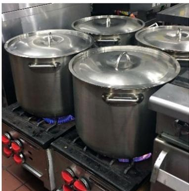
**Replacement stock pot ranges with finned-bottom pots for improved heat transfer.**
